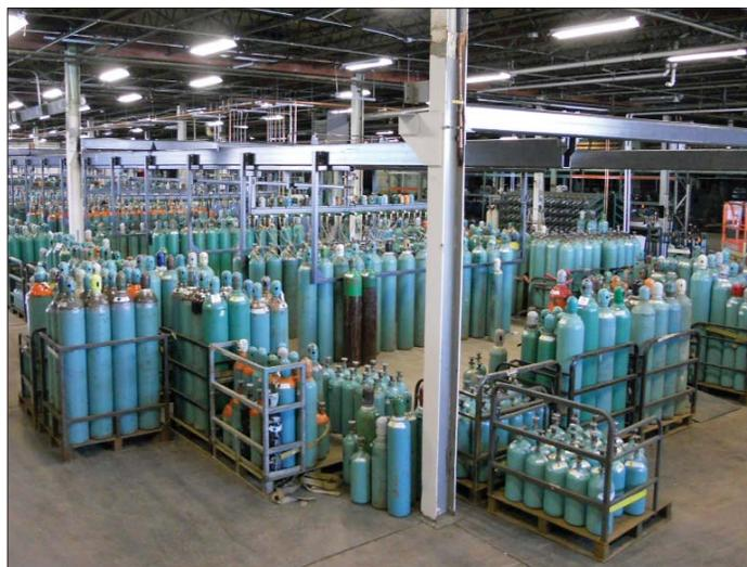
New Haun Specialty Gases plant boasts a 120 x 20-foot fill island with traversing manifolds.
